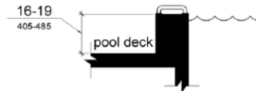
Figure 1009.4.2 Transfer Wall Height
